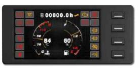
Interactive instrument: The instrument adopts 4.0-inch color LCD display with four interactive buttons, and has one CAN bus communication function. The communication protocol is compatible with CANopen and SAE J1939 standards.
