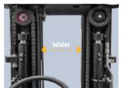
The developed front lifting cylinders with smaller outer diameter give the operator superior forward visibility.
