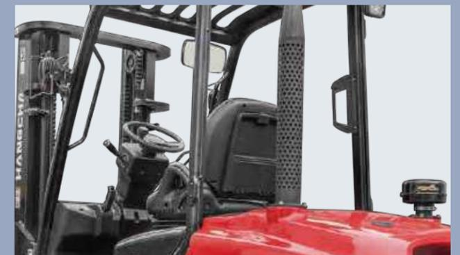
4. The new design mast provides broad forward visibility due to the longer distance between inside mast.
