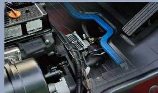
1. In addition to rubber damper between frames and steering axle, compound engine damper and full floating power train achieve flexible connection between frames and driving system, as a result, traveling vibrations and vibrations from the driving system are significantly reduced.
