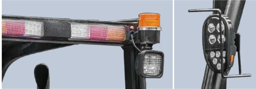
The new efficiency lighting system employs LED illuminant and new type reflector to reduce energy consumption, improve significantly illumination performance and prolong work time.
